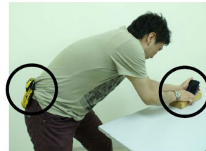
Figure 6. A plane attached to a smartphone and a smartphone attached to his waist
